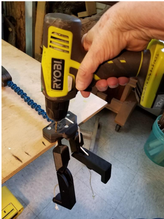
Drill a 9/64" hole through the back of the pelvis into the ball at the head of the femur 3/4" deep.
