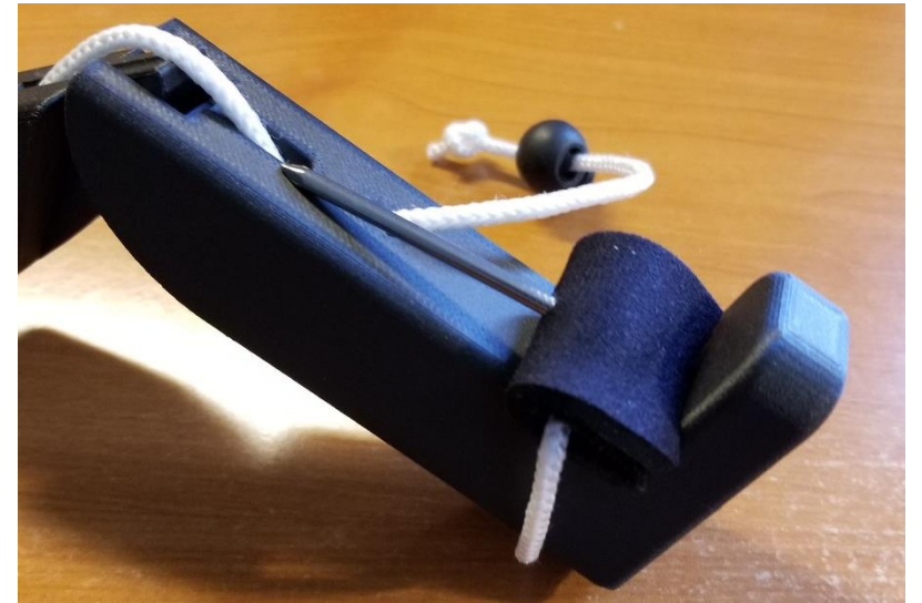
Pin can be a #6 nail. To make the nail easier to handle and keep up with, I put it through a small rectangle of Velcro accepting neoprene, tied a 7" long loop of string and held together with doublesided hook Velcro. The string allows the pin to slip over a foot for a holding place until needed.
